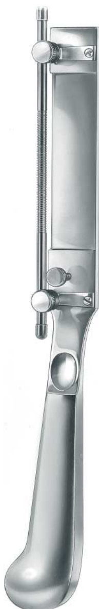
Schink SIT-01-111-30 30 cm adjustable from 0.1 to 2.0 mm
